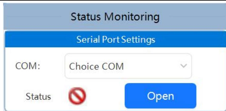
(4) After opening the serial port, the software will automatically read the driver's internal parameter settings for the first time. If communication fails, "Communication Fault" or "Failed to Read Parameters" will be displayed in the lower-left corner. Successful communication is determined by whether the driver parameters are read. If not, please check the hardware connection.
